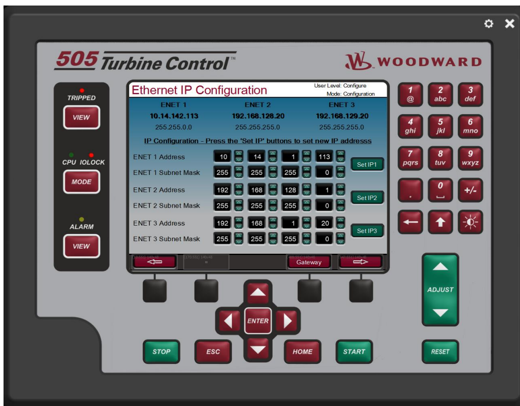
Figure H-1. Configuration/Communications Screen
